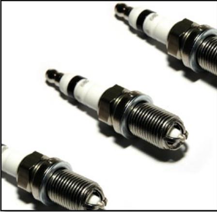
The spark plugs in a petrol engine are required to ignite the air-fuel mixture. However if the spark plugs are worn or not functioning correctly, the engine will misfire and some fuel will remain unburned. An engine which is misfiring wastes fuel, performs poorly and produces higher emission levels. Regular spark plugs should be replaced every 30,000 miles. Vehicles with distributors require additional ignition system maintenance.
