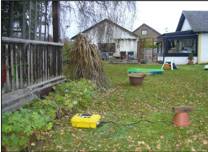
Figure 5.55: Photograph of Vibration Monitoring Equipment at Station House, Station Road, Kincardine
