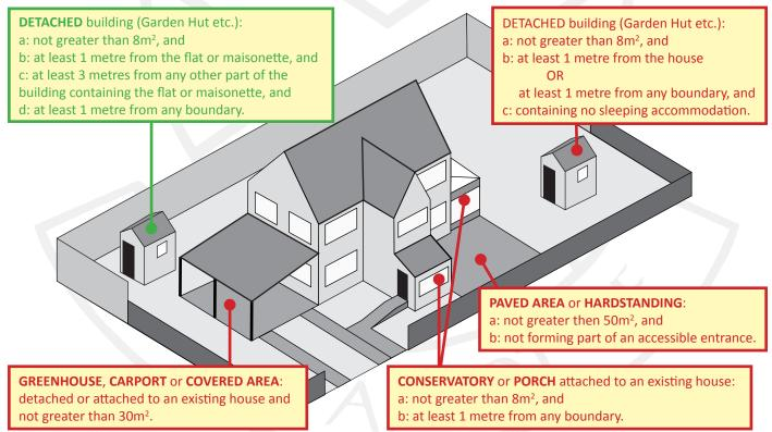
Exempt work may require that alterations are made to an existing building in order to maintain the level of compliance with the building regulations (for example; where it is intended to construct a porch over an accessible entrance then a new accessible entrance is required). In some circumstances (for example; where a new opening is formed between a dwelling and an exempt conservatory) a building warrant shall be required. July 2009
